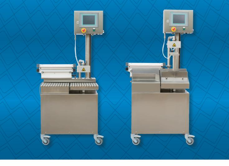
The **HOT-FILL DOS 2** ensures quick and precise dispensing of liquid food products. Soups, sauces and mashed potatoes are filled into bags and containers effortlessly. The built-in scale ensures that weighing of the product happens in one and the same workflow saving time in the kitchen. Changing the filling process from bags to containers only takes a few moments. Simply remove the bag holder, fit the roller track and the HOT- FILL DOS 2 is ready.
